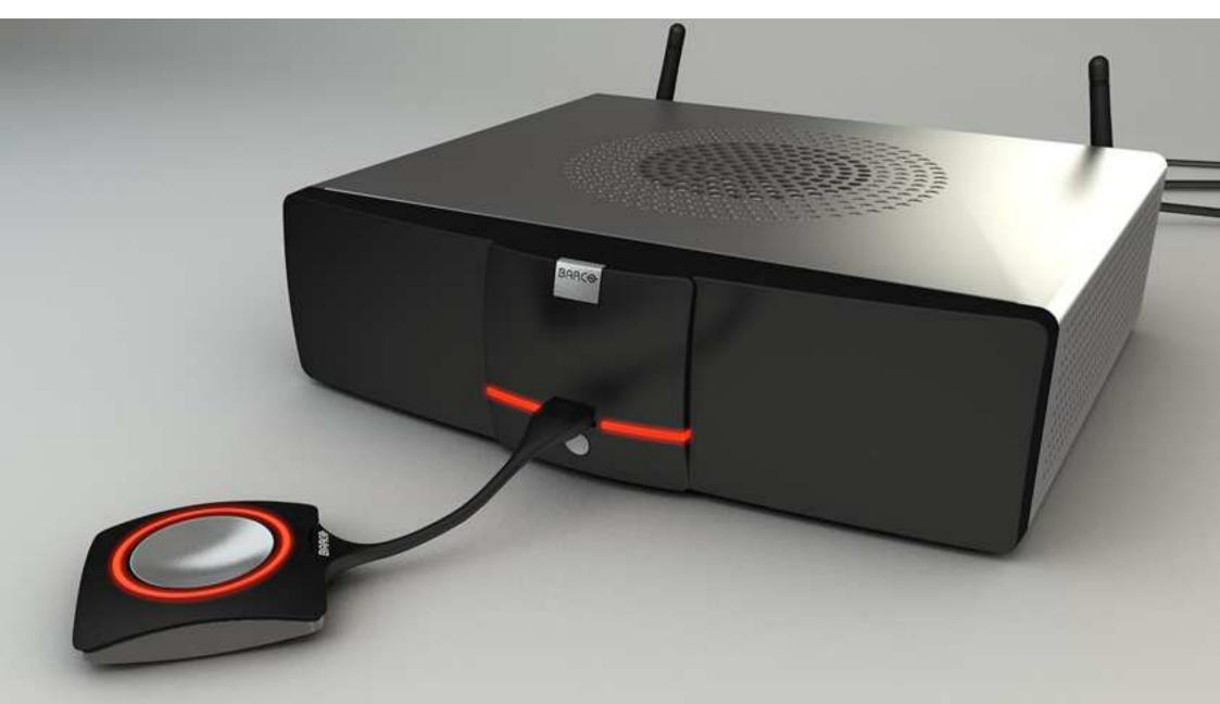
Pairing the dongle with the base unit
